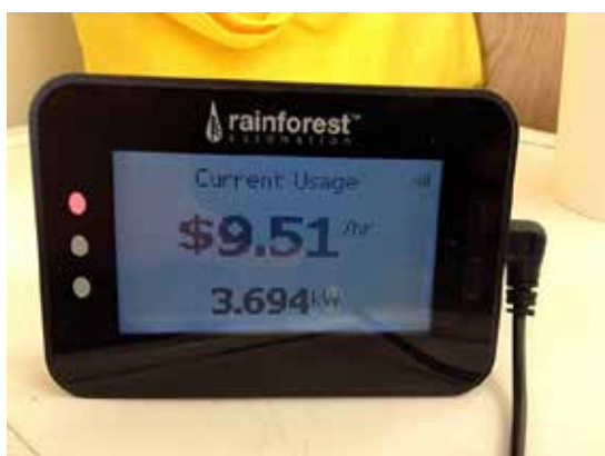
Electricity monitoring units allow residents of Jean Marie River to see their energy use in real time.
