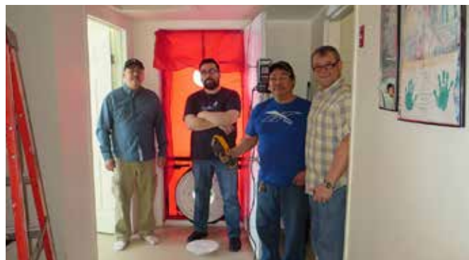
Conducting a blower door test in a home in Arviat.
