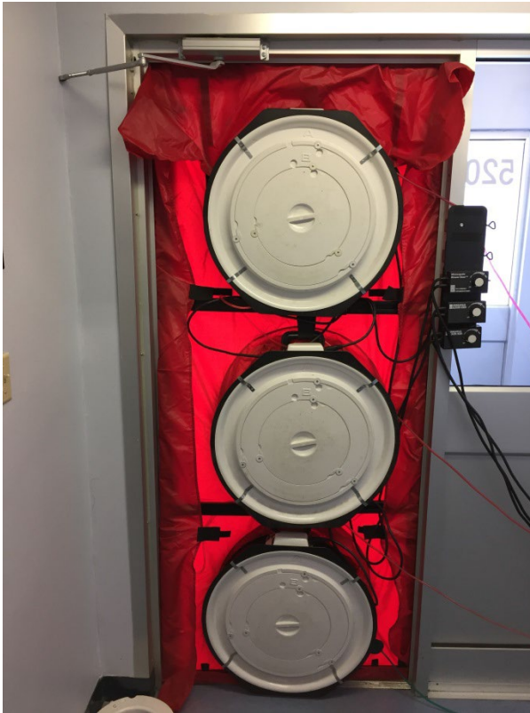
A blower door. Three-fan systems can be used in larger buildings, while a single-fan system would be used in a home or other smaller building.
