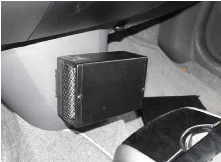
Electric cabin pre-heater used in Manitoba
