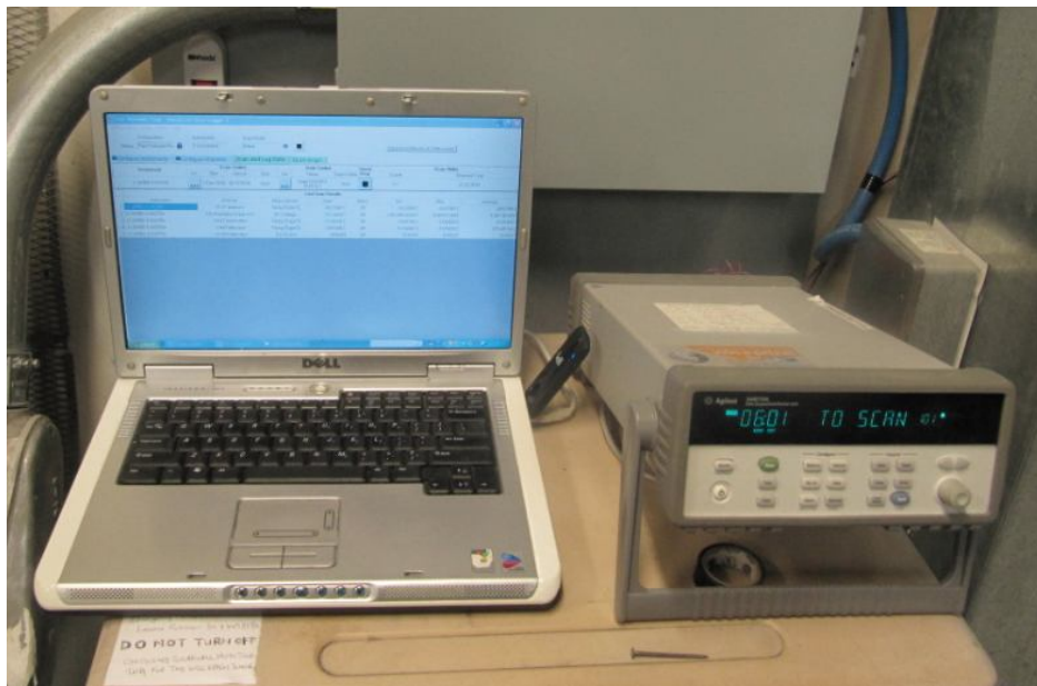
Figure 6. The Monitoring Laptop and Agilent Data Acquisition system for all new sensors
