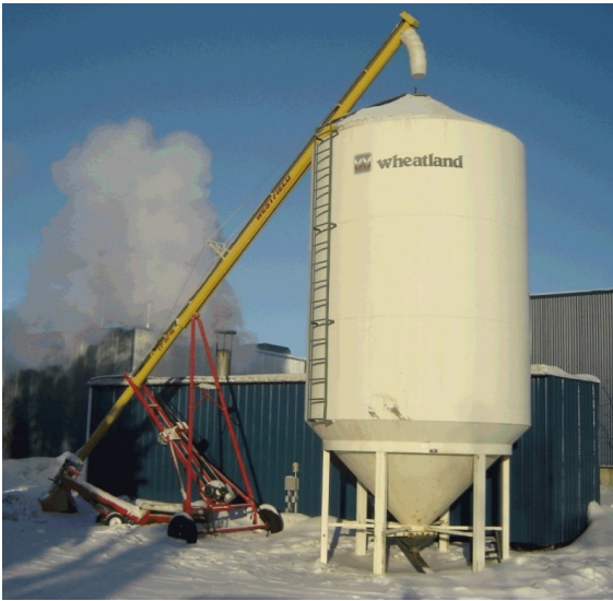
Left Photo: AEA. Welded steel plate silo. This 40t silo is 8.2m tall, diameter of 3.7m Right Photo: AEA. Bolted corrugated steel sheet silo. This 55t silo is 8.2 m tall, diameter of 4.3 m
