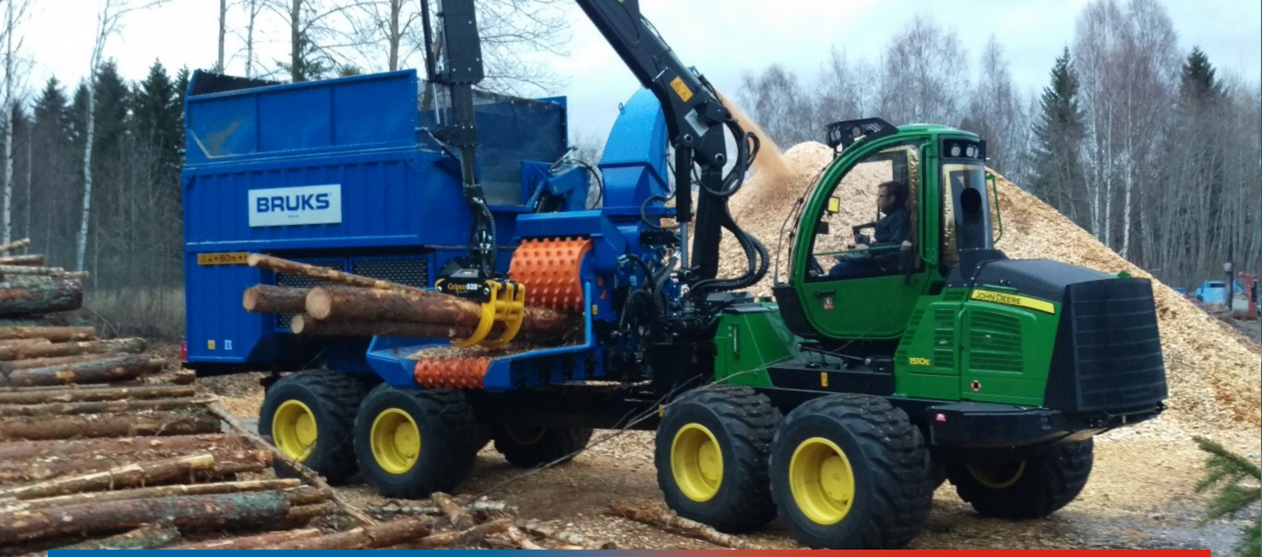
Forwarder mounted mobile chipper chipping at terminal
