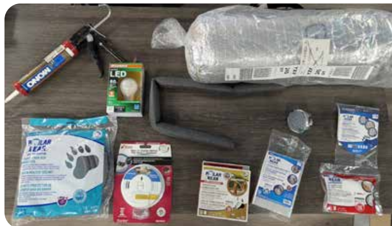
Materials used for the Home Winterization Walk-Through project include caulking, LED light bulbs, hot water tank insulation blankets, pipe insulation, a variety of weatherstripping, smoke detectors, low-flow shower heads and window plastic.
