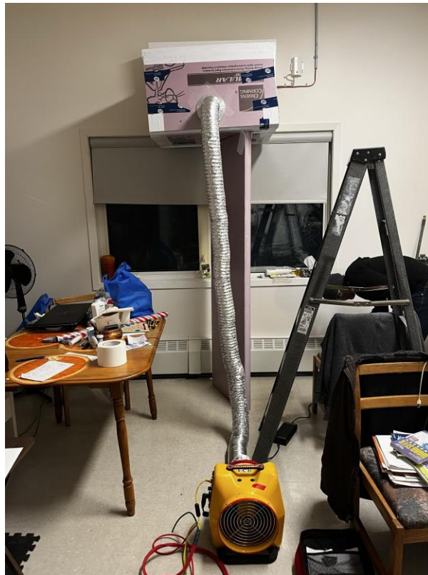
Figure 2.3 – Example of volumetric flow measurement apparatus mounted to a ductless mini split heat pump indoor unit.
